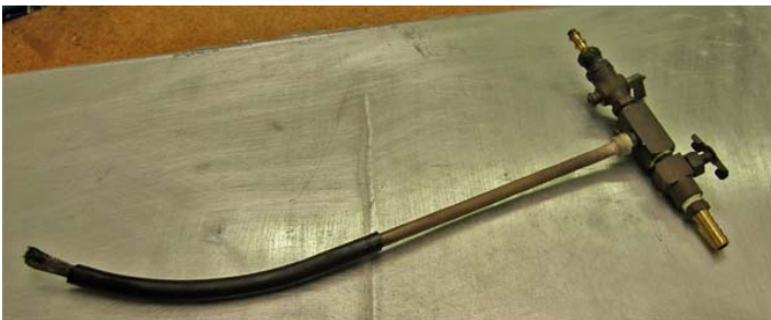
Fuel outlet line as designed by Catalina. Note the screen—rolled up and stuffed into the end of the rubber hose. This is the part that finally plugged and cut off all fuel to the
